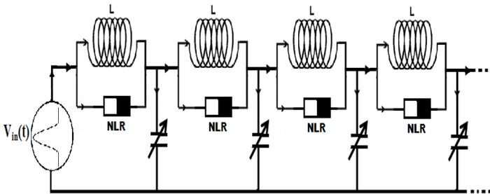
**Figure 1.** Schematic representation of the lumped nonlinear transmission line under consideration. Each cell contains the nonlinear capacitor  $C(V)$  in the shunt branch which induces the standard nonlinearity, the linear inductor  $L$  and the Nonlinear Resistance (NLR) introducing the linear dispersion and nonlinear diffusion, respectively, in the network.
