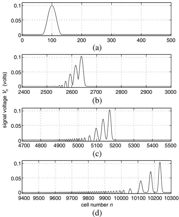
**Figure 6.** Propagation along the non dissipative NLTL of the compact electrical pulse signal. (a) Initially the width of this signal voltage centered at cell 100 is two times larger than that of the exact compact signal exhibited by this network (17), i.e.,  $L = 2L_c$ ; subplots (b), (c) and (d) show its decomposition at given dimensionless times of propagation:  $\omega_0 t_0 = 2575$ ,  $2\omega_0 t_0$  and  $4\omega_0 t_0$ , respectively.
