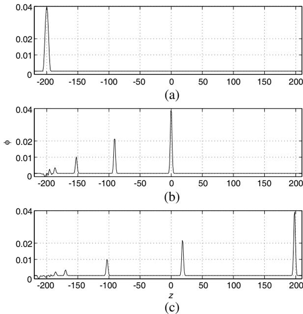
**Figure 4.** Propagation of a compact wave. (a) Initially the width of the wave-packet is two times larger than that of the exact compact wave (43), i.e.,  $k = k_c/2 = 0.25$ ; subplots (b) and (c) show the decomposition of this wave-packet at given dimensionless times of propagation:  $T_0 = 4875$  and  $2T_0$ , respectively.
