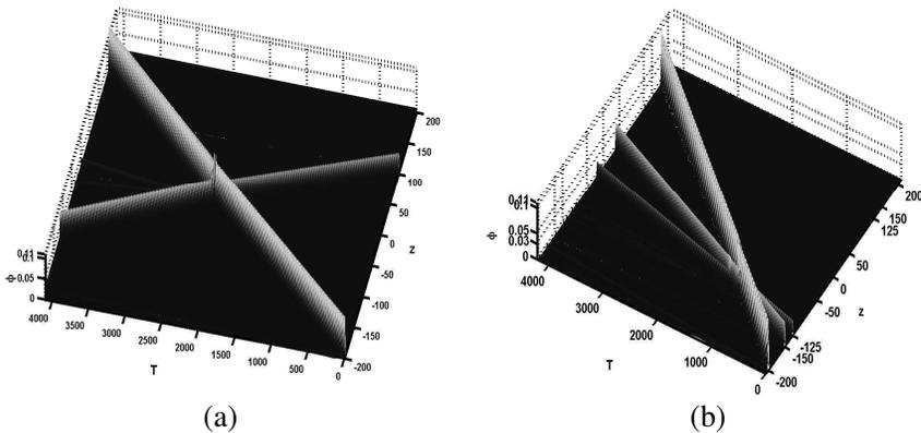
**Figure 3.** Propagation and head-on collision between (a) two and (b) three compact solitary waves. Initially these waves are localized at positions  $z = -200$  and  $z = 100$  for the first case and for the second case at the positions  $z = -200$ ,  $-150$  and  $-125$ . In this latter case, pulses have different amplitudes  $A_0 = 0.1$ ,  $0.05$  and  $0.03$  propagating in the same direction. The waves maintain their shape after collision.
