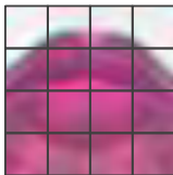
Fig. 3. Example of a 4x4 grid employed for the computation of local descriptors. The patch size is a square of 8 pixels.
