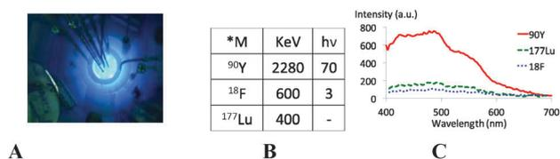
Fig. 1 (A) Cherenkov radiation (CR) observed in a nuclear reactor. (B) Correlation between the intensity of the emitted CR, the energy of emitted β<sup>-</sup>/β<sup>+</sup> particles, the reported yield in photons per decay,<sup>8,15</sup> and the luminescence intensity. (C) Spectroscopic detection of CR emitted by [<sup>90</sup>Y]-YCl<sub>3</sub> (16.2 MBq), [<sup>18</sup>F]-FDG (46.5 MBq), and [<sup>177</sup>Lu]-LuCl<sub>3</sub> (318.3 MBq) in saline buffer (zoom in the 400–700 nm region).
