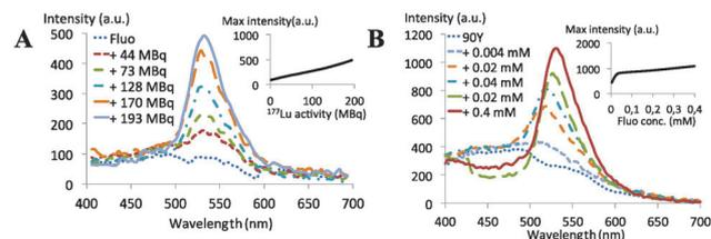
**Fig. 4** (A) Increase of the intensity of the fluorescence emission signal of fluorescein (0.4 mM) is a function of the quantity of [ $^{177}\text{Lu}$ ]- $\text{LuCl}_3$  (*i.e.* radioactivity). Inset: monitoring of the increase at  $\lambda_{\text{em}}$  of fluorescein (526–529 nm). (B) Increase of fluorescence upon addition of fluorescein at constant activity (6.9–9.5 MBq). Inset: fluorescence monitored at maximum intensity (508–526 nm) upon addition of [ $^{90}\text{Y}$ ]- $\text{YCl}_3$ .
