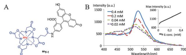
**Fig. 5** (A) Structure of  $^{90}\text{Y-1}$ : a fluorescein-DOTA conjugate with a built-in radionuclide (synthesis in Fig. S5, ESI†). (B)  $^{90}\text{Y-1}$  fluorescence emission upon inter- and intramolecular CRET processes at various concentrations (and constant activity, 9 MBq). Inset: monitoring of the increase at  $\lambda_{\text{em}}$  of fluorescein (520 nm).
