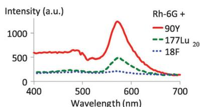
**Fig. 3** The intensity of the rhodamine 6G (0.4 mM) fluorescence emission is a function of the energy of the particle emitted during the radionuclide decay: 400 keV ( $^{177}\text{Lu}$ , 180 MBq), 600 keV ( $^{18}\text{F}$ , 61.5 MBq), and 2280 keV ( $^{90}\text{Y}$ , 9.5 MBq), *i.e.* the amount of emitted optical CR photons.
