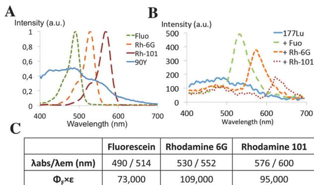
**Fig. 2** (A) Position of the absorption  $\lambda_{\text{max}}$  of fluorophores with respect to the CR emission spectrum. (B) Fluorescence emission of fluorophores (0.4 mM) upon CRET (and CR radiation remaining at the bottom of the spectrum) ( $^{177}\text{Lu}$  180–190 MBq). Working solution: 0.15 M (0.9%) NaCl solution/MeOH (or 0.1 M NaOH solution) 6 : 4 vol., at RT (see ESI†).
